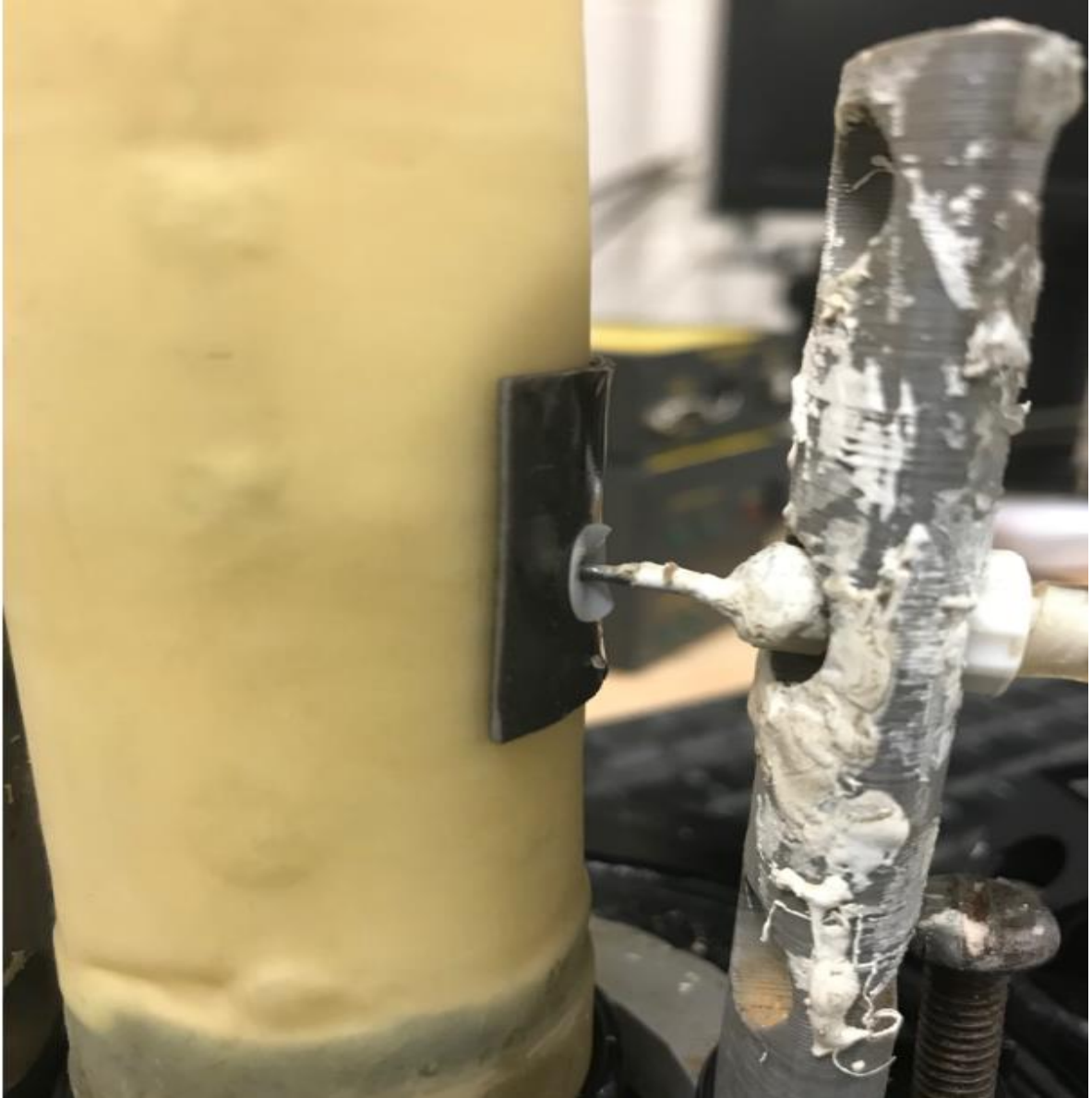
Figure 19. Setup for insertion of the needle at mid-height
