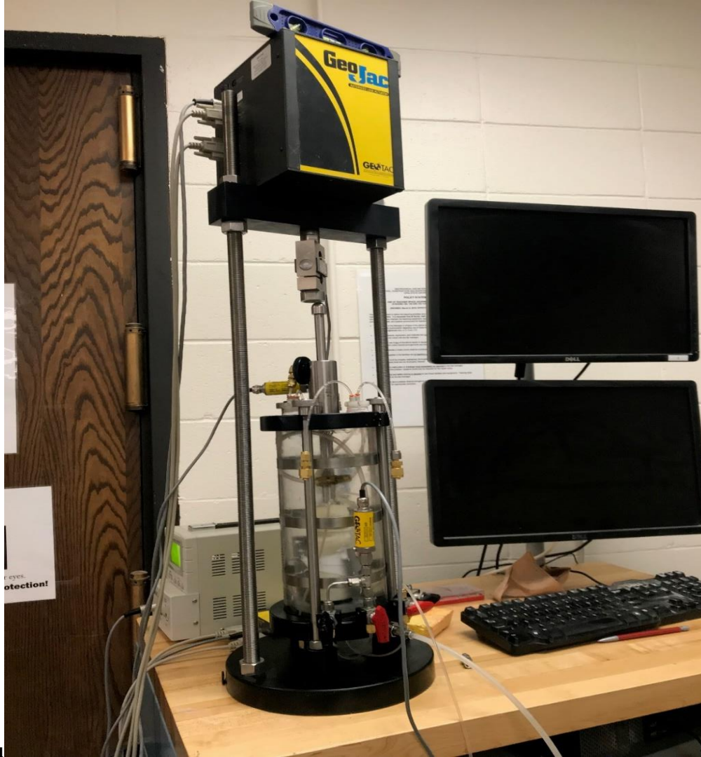
Figure 15. Geotac Monotonic Triaxial testing setup
