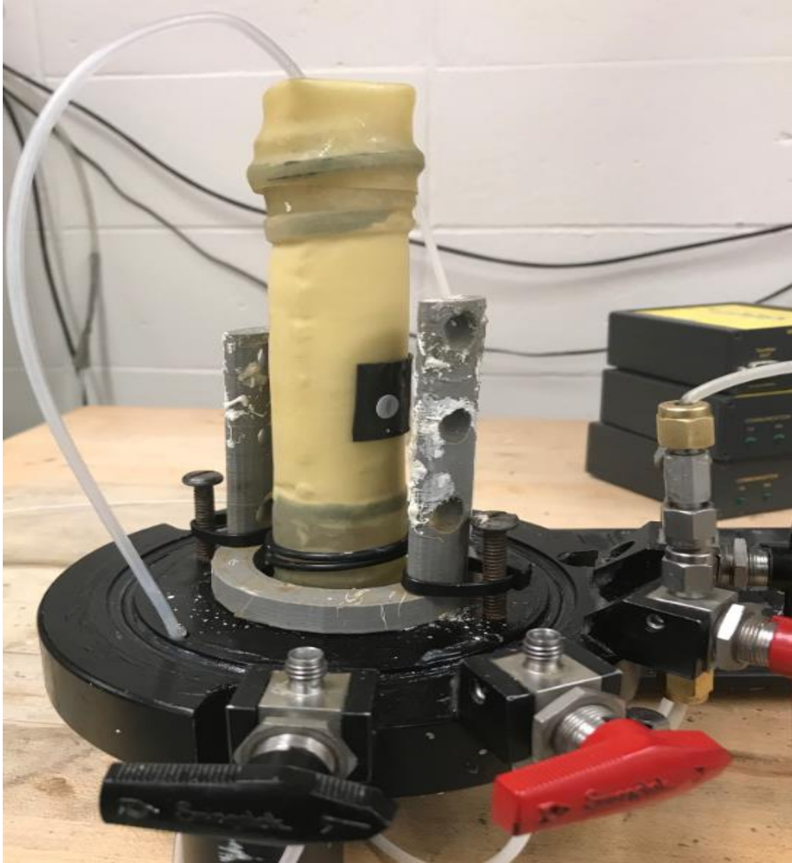
Figure 18. Setup for measuring mid-height PWP
