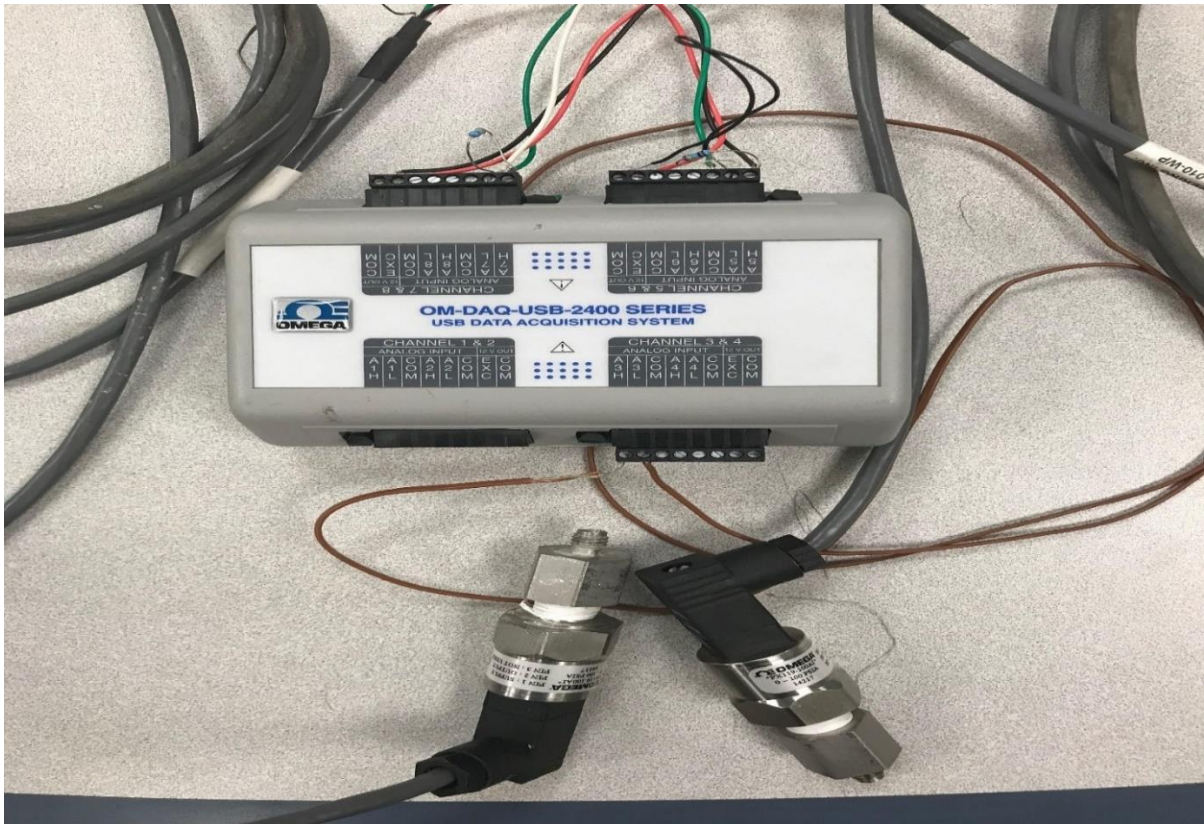
Figure 21. Data acquisition system and pressure transducer
